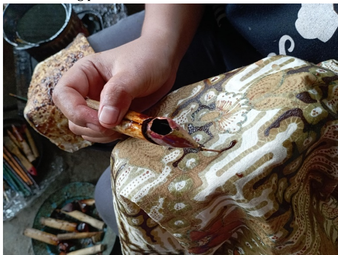
Figure 3. The Process of Sticking The Hot Night Using Canting to Protect The Fabric From Being Exposed to Coloring Materials.
